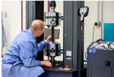
State of the art testing equipment provides immediate feedback on large format printed samples, including tensile, flexural and compressive properties. This in-house capability provides the opportunity to validate our optimized print parameters and add speed to our customers' application development process.
